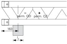
perm.  $A_n = 16.0 \text{ kN}$ perm.  $Q_D = 14.0 \text{ kN}$ perm.  $Q_Z = 13.0 \text{ kN}$
