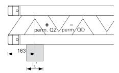
perm.  $A_{m} = 13.0 \text{ kN}$ perm.  $Q_{Z} = 13.0 \text{ kN}$
