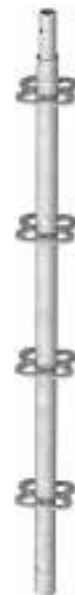
The Standard UVR is available in lengths of 50 cm to 400 cm (in 50-cm or 100-cm increments). The integrated 50-cm rosette spacings match the logical grid dimensions.
