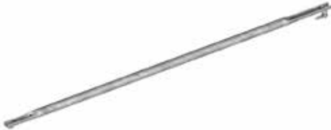
The Ledger Brace UBL is available in lengths from 100 cm to 300 cm (in 50-cm or 25-cm increments). It is attached using holes in the ledgers.
