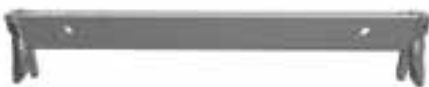
The lightweight UH Ledger is available in lengths ranging from 25 cm to 400 cm – with 25-cm or 50-cm increments. Use of the strengthened Ledger UHV is recommended for spans of 1.50 m or more.
